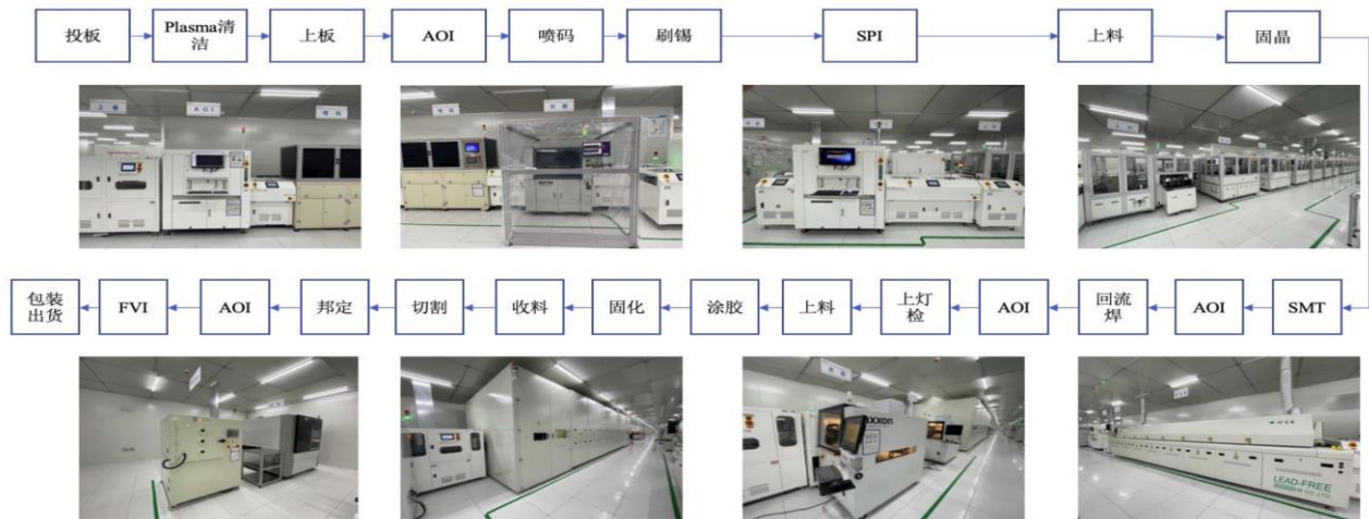
图20：Mini LED 背光模组相较于传统显示模组工艺更加复杂
